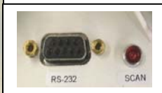
Figure 2: Serial cable (left) and the WeatherHawk serial port in which the serial cable male connector connects. A dust cover must be removed from the WeatherHawk RS-232 port before connecting the cable.
